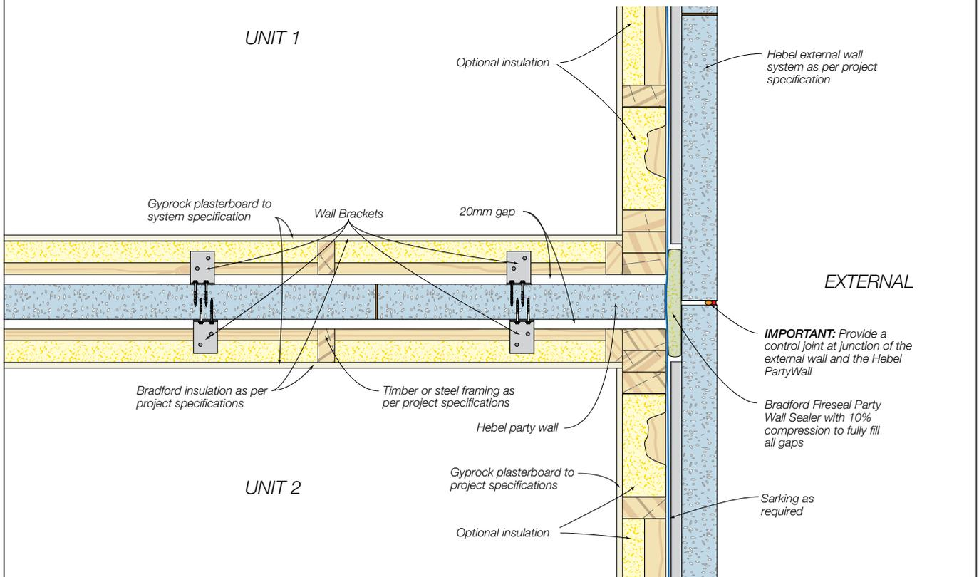
Figure 3.3.6.2 External wall corner junction for PowerPanel<sup>XL</sup> Intertency Wall System
