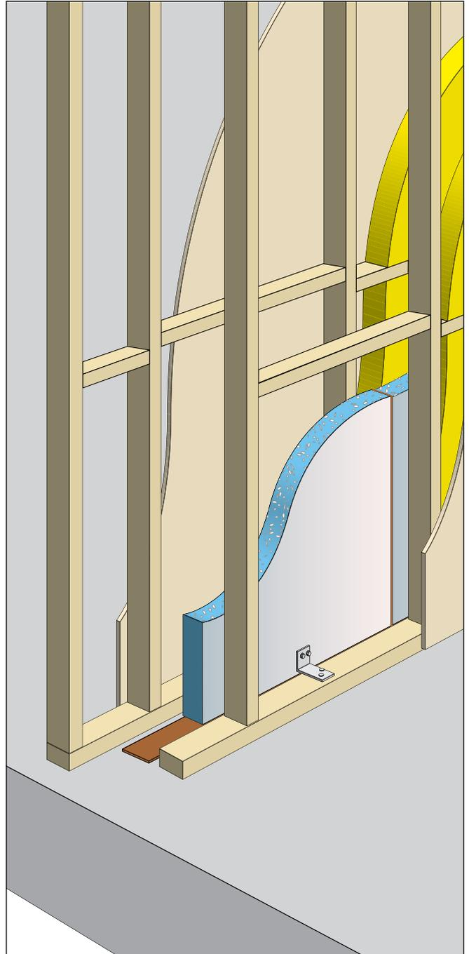
**Hebel PowerPanel<sup>XL</sup> Intertenancy Wall System for load bearing and non-load bearing intertenancy / party walls in low rise multi-residential projects. This wall configuration consists of Hebel (non-load bearing) PowerPanel<sup>XL</sup> panels installed vertically and secured to the structural load bearing frame. The system utilises an aluminium bracket system which provides the wall with a discontinuous construction for acoustic performance.**
