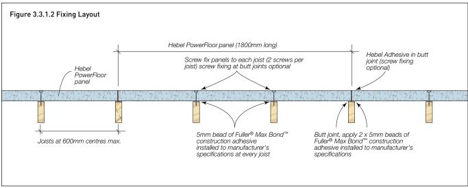
Figure 3.3.1.3 Fixing of Hebel PowerFloor Panel to Timber Joists
